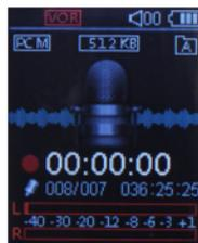
(Note: When choosing VOR Mode, it will end recording when the sound source level is lower than the preset VOR sensitivity, and recording timer will also be stopped. When the recording sound source exceeds the minimum level again, the device will continue to record, and it can be turned on or off as demanded.
