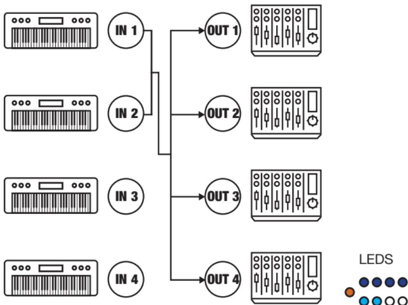
The MIDI merge function allows you to mix data from the Input 1 and Input 2. The mixed data is then distributed to all four outputs.
