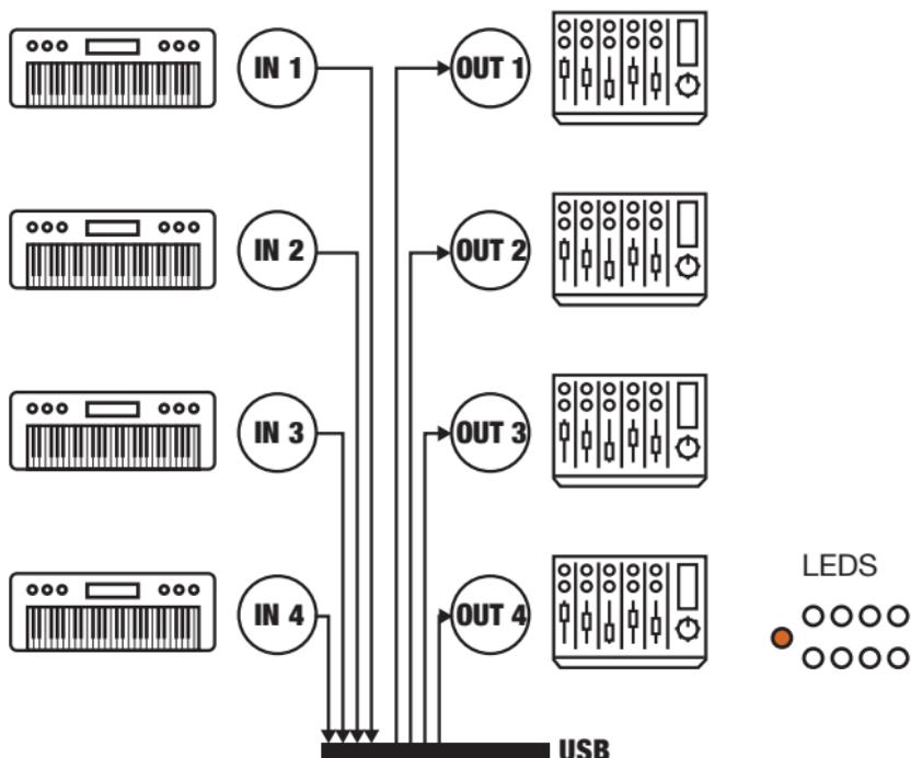
When you select this mode, TIE 4i4o will be working as a basic MIDI interface. This is the normal operation mode. MIDI signals from your sequencer applications will be sent out and can be recorded via the in and outputs of TIE 4i4o. When the device is connected with computer's USB port, it is in the USB mode and the orange LED will light.
