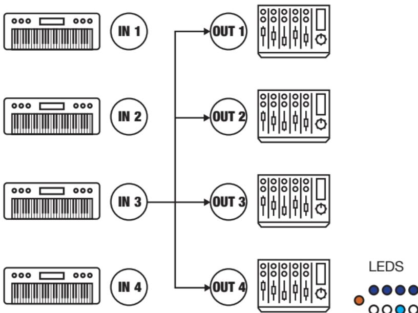
In this mode, input 3 is connected to the 4 outputs.
