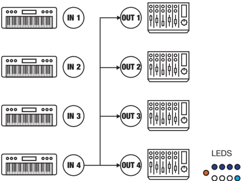
In this mode, input 4 is connected to the 4 outputs.
