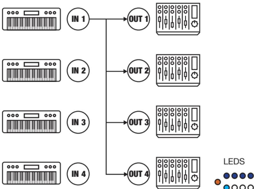
In this mode, input 1 is connected to the 4 outputs.
