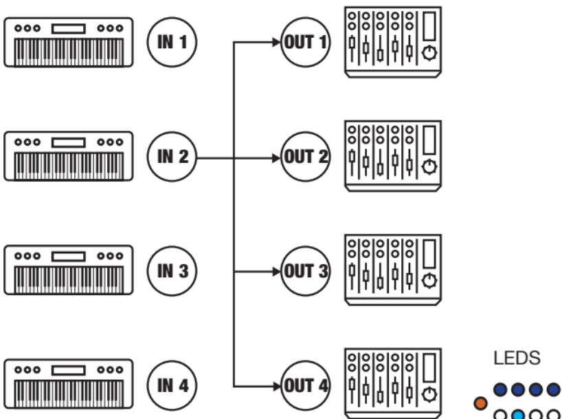
In this mode, input 2 is connected to the 4 outputs.
